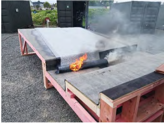
Photo 30: Flame penetrating through membrane on the roll. Notable is the white puffing smoke similar to that observed at the NZICC.
