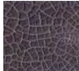
Photo 43: Example of crocodiling visible on base sheet after long term exposure to UV.
