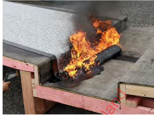
Photo 31: Fire developing beyond the roll to the vertical gutter surface and beginning to extend to the horizontally laid Cap Sheet representing the main roof surface. Smoke is becoming black.
