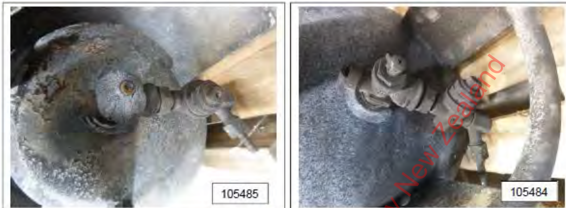
Figure 4: Valves of both cylinders in as found condition
