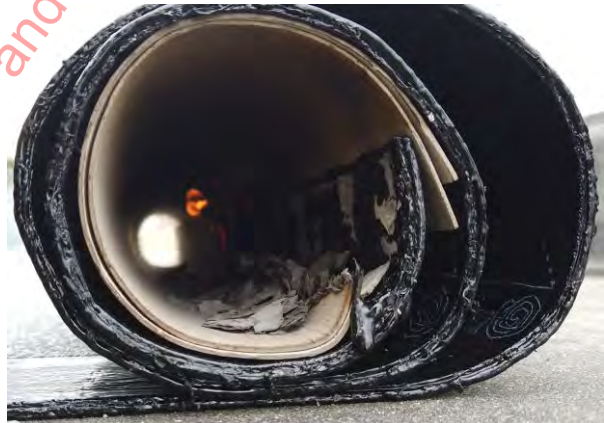
Photo 29: Gradual smouldering tracked inside the roll with occasional flickering flame returning to smouldering.
