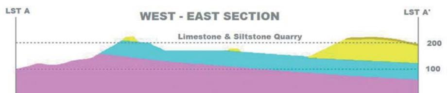
Cross section west-east: this shows a section through the quarry looking from the south towards the north. The gently sloping floor of the quarry would be rehabilitated for use as general farmland.
