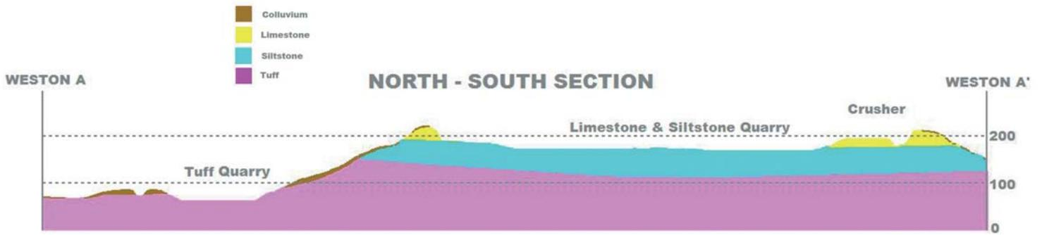
Cross section north-south: this shows a section, viewed from the west looking east, through the quarry as expected at year 30. Note the tuff quarry at the northern (left) end of the section, and the dish-shaped area of the quarry. The Whitstone limestone escarpment would remain and is shown as the yellow areas. Note that when viewing cross-sections, the escarpment in front of the cross-section is 'invisible' so as to allow a view into the quarry.
