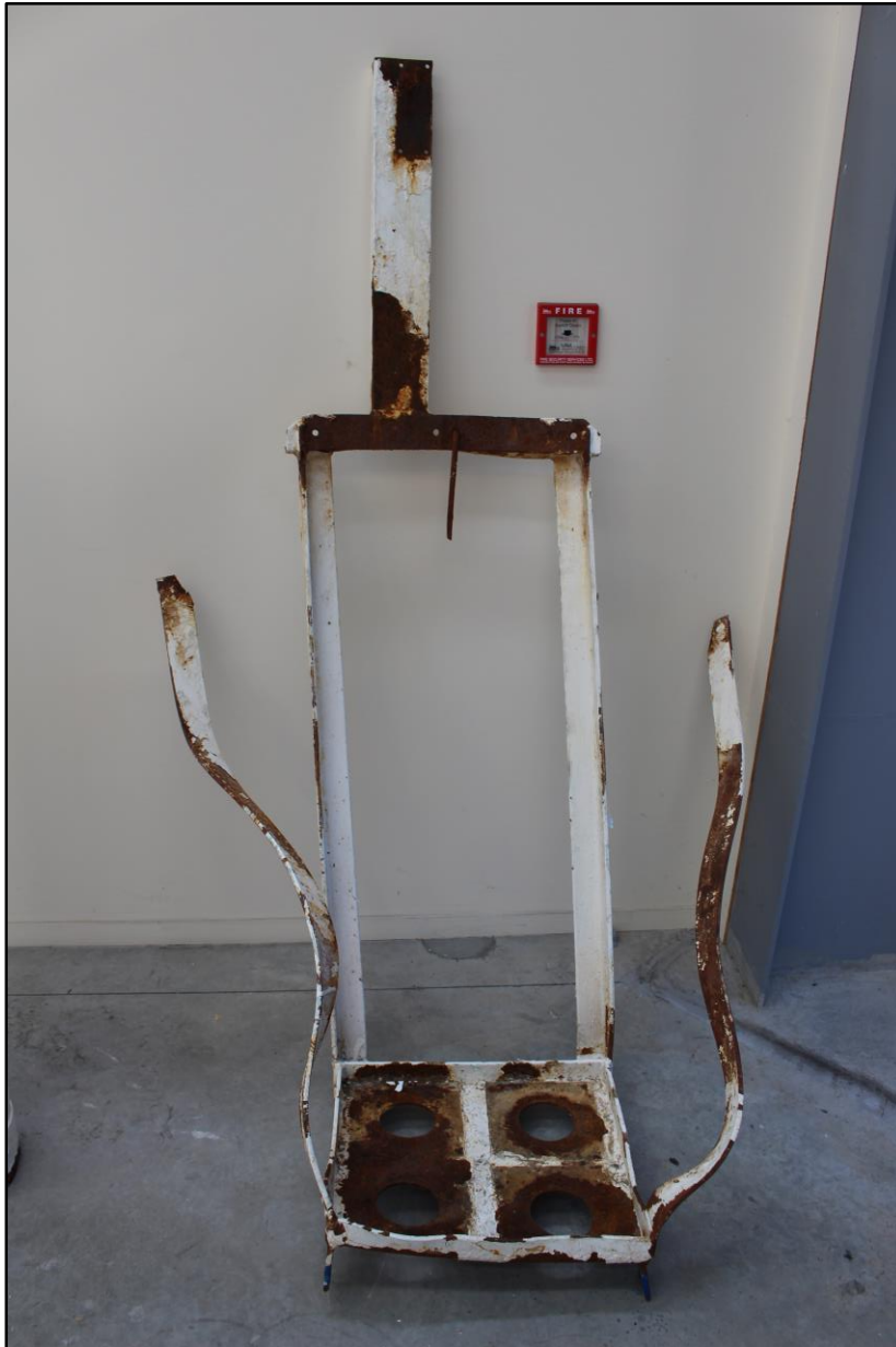
Figure 2 Damaged storage frame that held the burst cylinder
