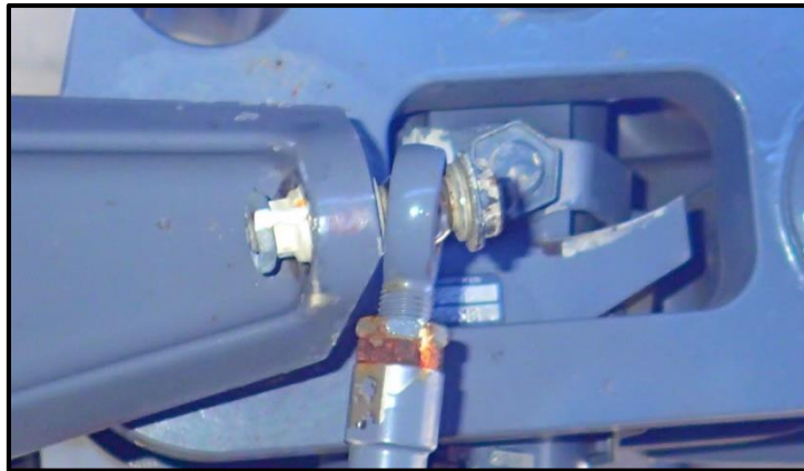
Figure 11 Contact between the pitch link and the pitch horn at the teeter limit (7.4 degrees)
