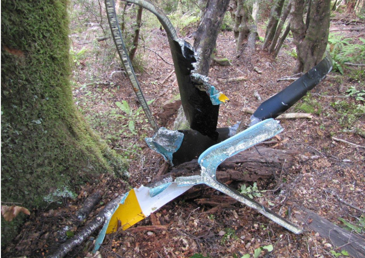
Figure 3 Main rotor as found
