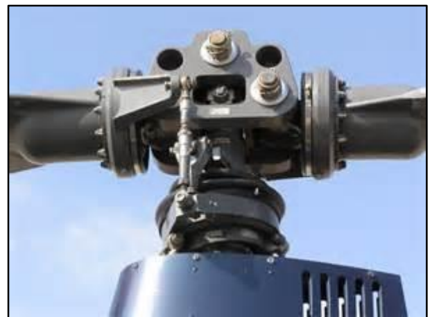
Figure 4 R44 pitch link input outboard of teeter hinge and inboard from coning hinge
