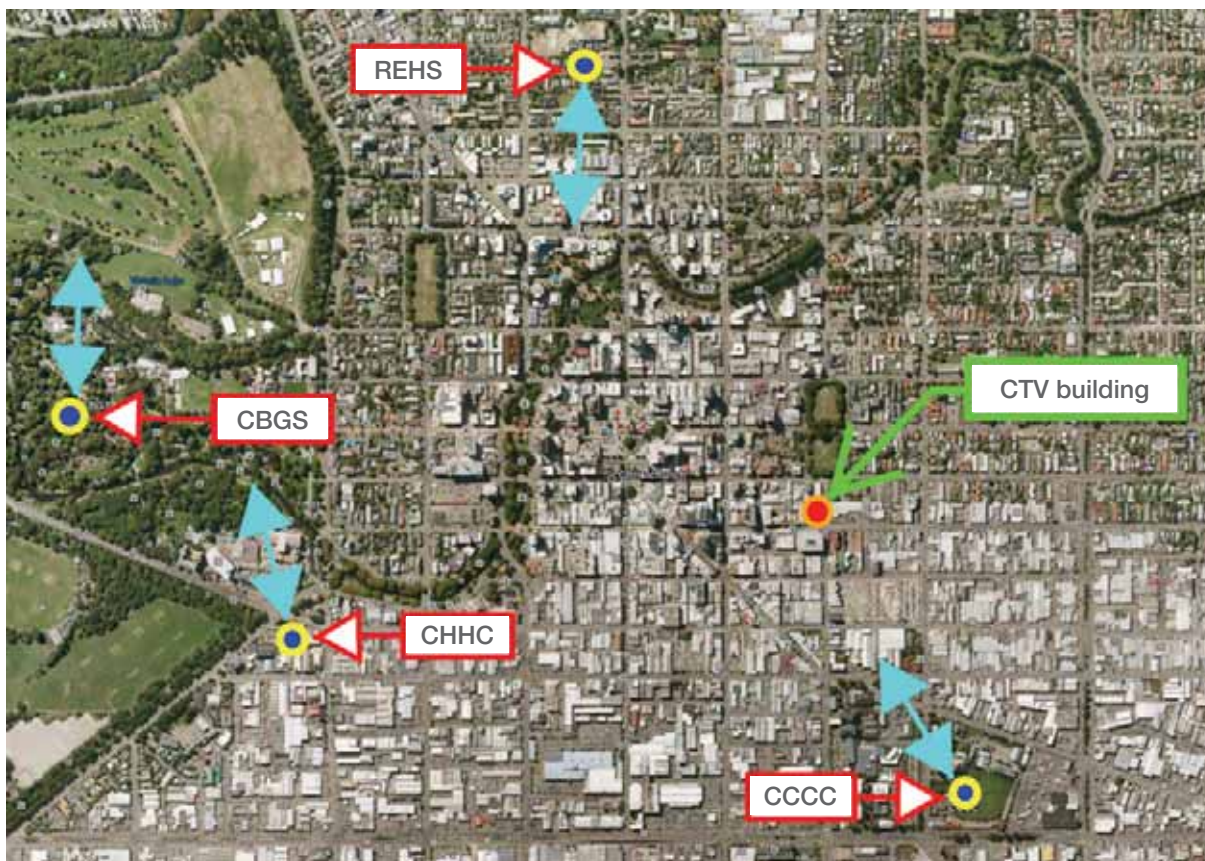
Figure 31: Location of seismic measuring stations and predominant direction of ground accelerations at the site of each location in the September earthquake. The location of the CTV site is also shown
