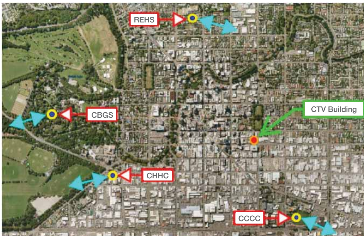
Figure 51: Location of seismic measuring stations and predominant direction of ground accelerations at the site of each location in the February earthquake. The location of the CTV site is also shown.
