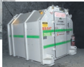
A six person portable refuge chamber.
