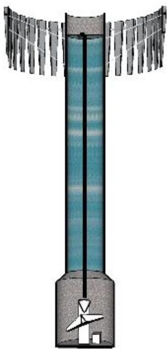
The gauges consist of two-metre high pipe filled with mono-propylene-glycol (an agricultural food supplement that also works as an antifreeze!). An overflow tube runs from the top of the pipe down to the base where it feeds into a normal rain gauge.
