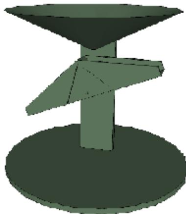
A standard rain gauge is made up of a funnel that guides rainfall onto one of two small buckets on either end of a see-saw.
