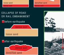
Approaches to bridges and stopbanks are particularly vulnerable. Roads, railway tracks and other structures built on fill
