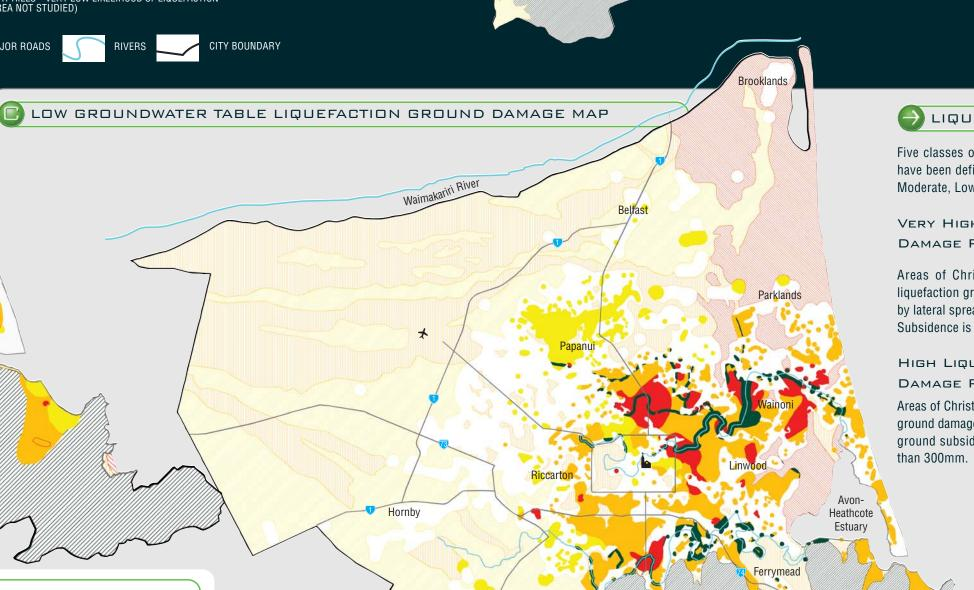
🕒 LIQUEFACTION GROUND DAMAGE POTENTIAL Five classes of liquefaction ground damage potential Moderate Liquefaction Ground have been defined for Christchurch - Very High, High, DAMAGE POTENTIAL Moderate, Low and No Liquefaction.
