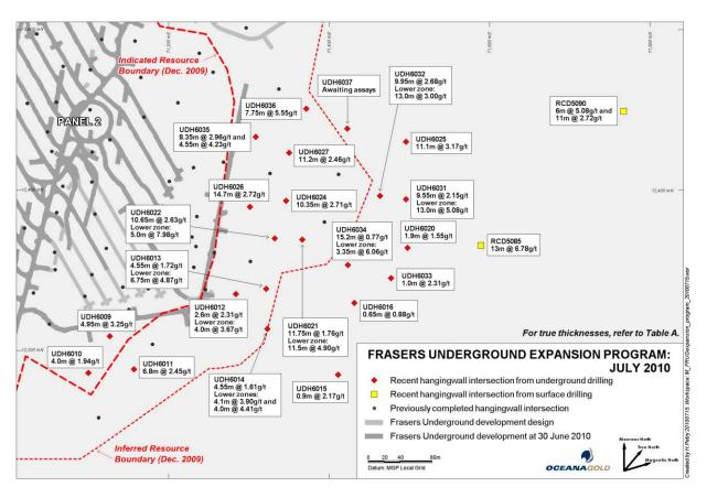
Diamond drilling from the underground exploration drive continues to infill gaps in the known mineral resources and is also testing for extensions to the north, south and southeast. Indications are that the Panel 2 mineralisation is likely to continue in these directions and may eventually join or extend beyond the intercepts recorded from the surface exploration holes RCD5085 and RCD5090 announced on 3 May 2010.
