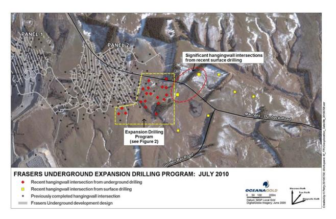
Diamond drilling from the underground exploration drive tested up to 250 metres east (down dip) of the current mine design (Figure 1) and extended out towards the significant surface drilling intercepts (RCD5085 and RCD5090) announced 3 May 2010. All holes completed to date successfully intercepted the main mineralised Hangingwall Shear structure.
