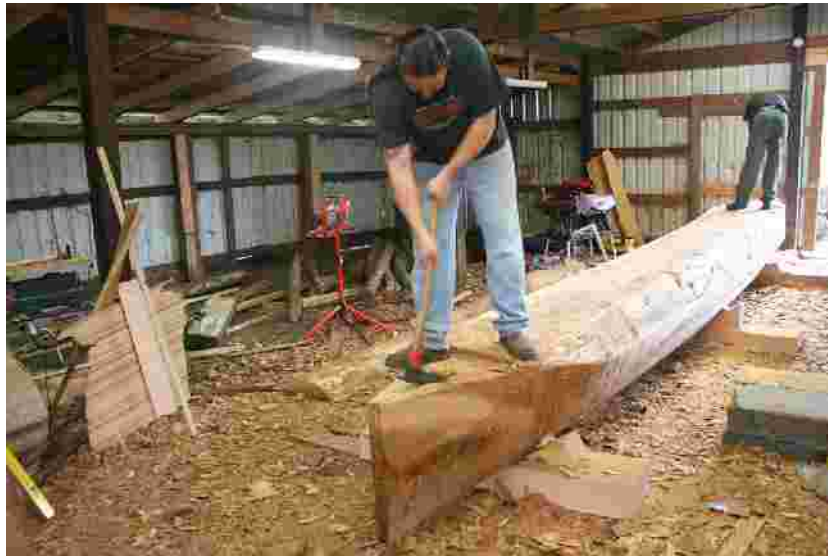
Canoe Builder Bobby Mercier adzing a canoe being built for Canoe Journeys 2009
