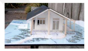
The children have come up with a design which utilises sustainably-harvested timber, a concrete floor to retain heat, natural light and ventilation, double glazing and pergolas on the west and north sides. Solar heating will be used to heat the nearby school pool, and rainwater will be collected from the roof for a native garden.
